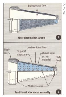
Fig. 4. Conventional filter screen, *A*, is an assembly of components, which adds cost to the structure. Moreover, support grid protects the screen from rupturing in only one direction of flow. One-piece filter screen machined from bar stock, *B*, is self-supporting, which prevents collapse in either direction, even when full pressure is applied to a completely clogged screen.
