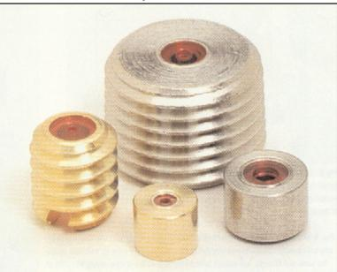
Fig.1. Close control of tight tolerances is essential to miniature components, because a deviation of 0.1301 in. allows 5% error for a 0.020-in. ID orifice. Rut if the orifice has an ID of only 0.005 in., that same 0.001 in deviation creates an error of 20%.
