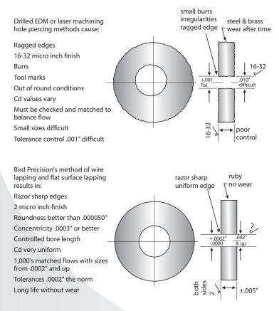
Many hydraulic engineers require balance flow in their systems. Therefore, in spool valves and servo valves where a shuttle oscillates back and forth between ports that contain an orifice, or in applications where two cylinders are required to lift in tandem with the same stroke, orifices with balance flow are critical.
