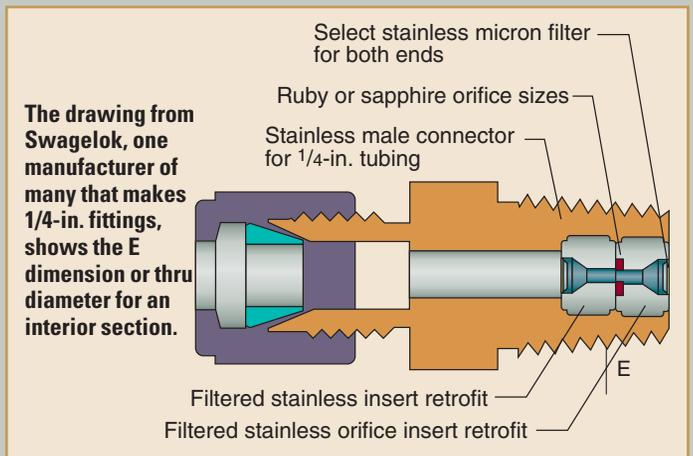
thousands are produced in each batch. Machined metal orifices, on the other hand, have burrs and out-of-round holes from drill wobble.
