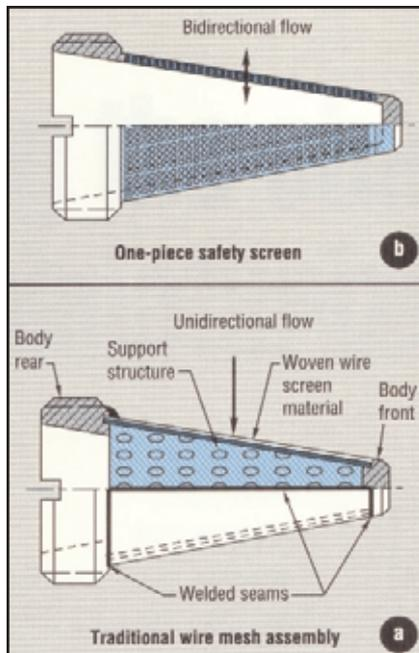
**Fig. 4. Conventional filter screen, A, is an assembly of components, which adds cost to the structure. Moreover, support grid protects the screen from rupturing in only one direction of flow. One-piece filter screen machined from bar stock, B, is self-supporting, which prevents collapse in either direction, even when full pressure is applied to a completely clogged screen.**
