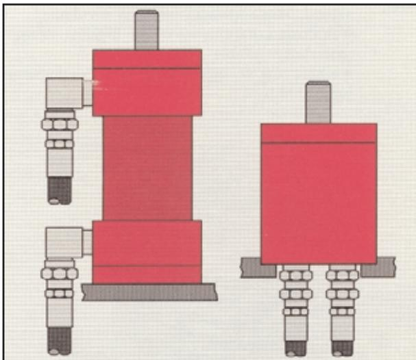
Fig. 2. Conventional double-acting cylinders, left, consume substantial space to accommodate fitting and hose at both head and cap ends. Bottom-ported cylinders, right, reduce the envelope by locating inlet and outlet ports at the cap end.
